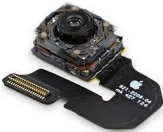
Largan makes only lenses. The complete camera module (see photo below of the module from the iPhone) is assembled by other manufacturers, a task that still requires some hand labor and offers tiny margins of 5% or less.
